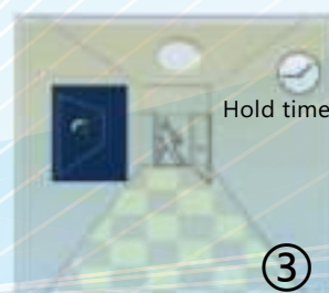
③ After the last detection, the light will be dimmed down to the stand-by dimming level (10%,30%,50%) after hold time
